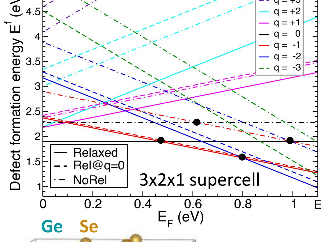
Defect formation energies as a function of **supercell size**: **convergence** is reached
