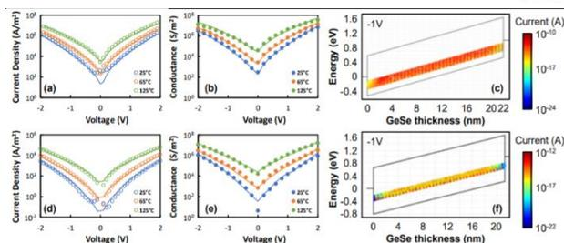
**Figure 2.** (a), (d) Current and (b), (e) conductance densities simulated (lines) and measured (symbols) at different temperatures on 20nm-thick (top row) TiN/Ge<sub>60</sub>Se<sub>40</sub>/TiN and (bottom row) TiN/Ge<sub>50</sub>Se<sub>50</sub>/TiN capacitors. (c), (f) Corresponding trap distributions as extracted by applying the proposed methodology.
